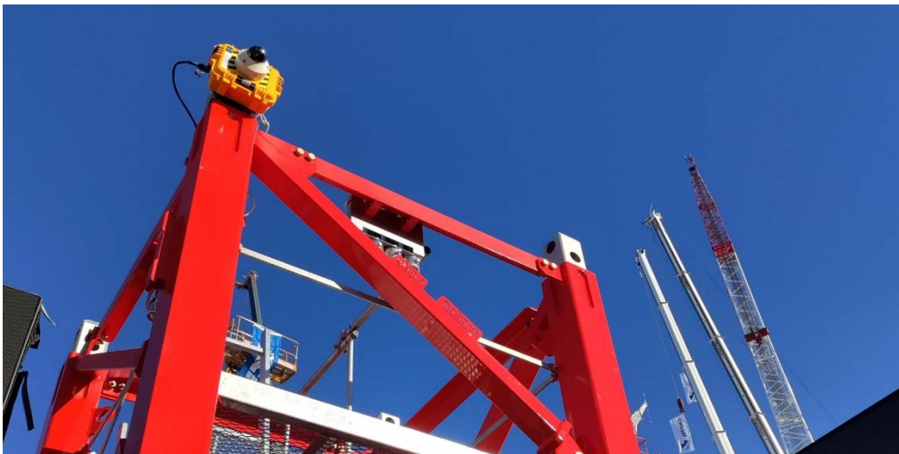
Frame mounted camera on equipment (Photo Courtesy HoistCam by Netarus)
